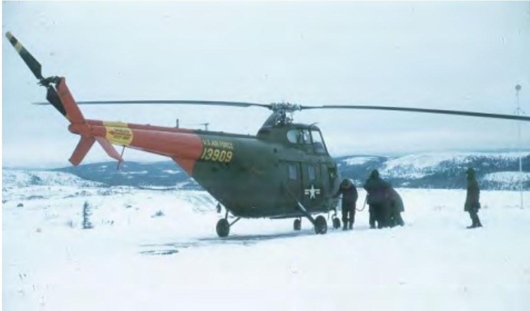
Photo 9: View during the refueling of helicopters in 1953. Note the helicopter is refueled using drum with manual pump.
