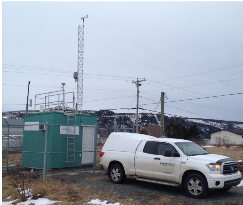
EnviroShelter for community monitoring Water, Air/Gas, Noise, and Meteorological Parameters
