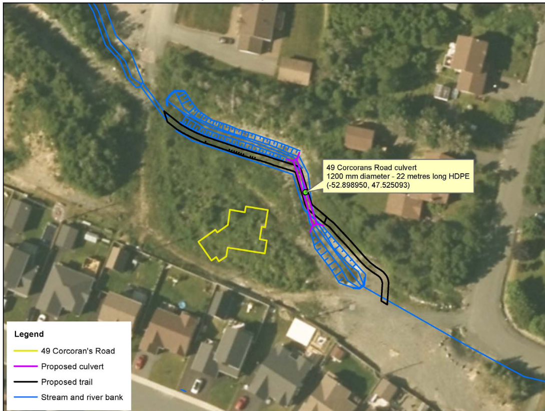
Pedestrian culvert installation along a trail at 49 Corcoran's Road, Paradise
