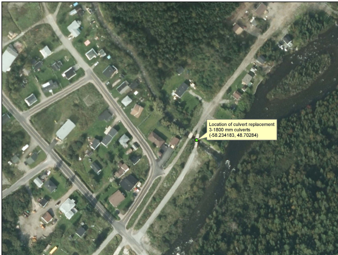
Replacement of 7A Brook Bridge with 3-1800 mm culverts in Gallants
