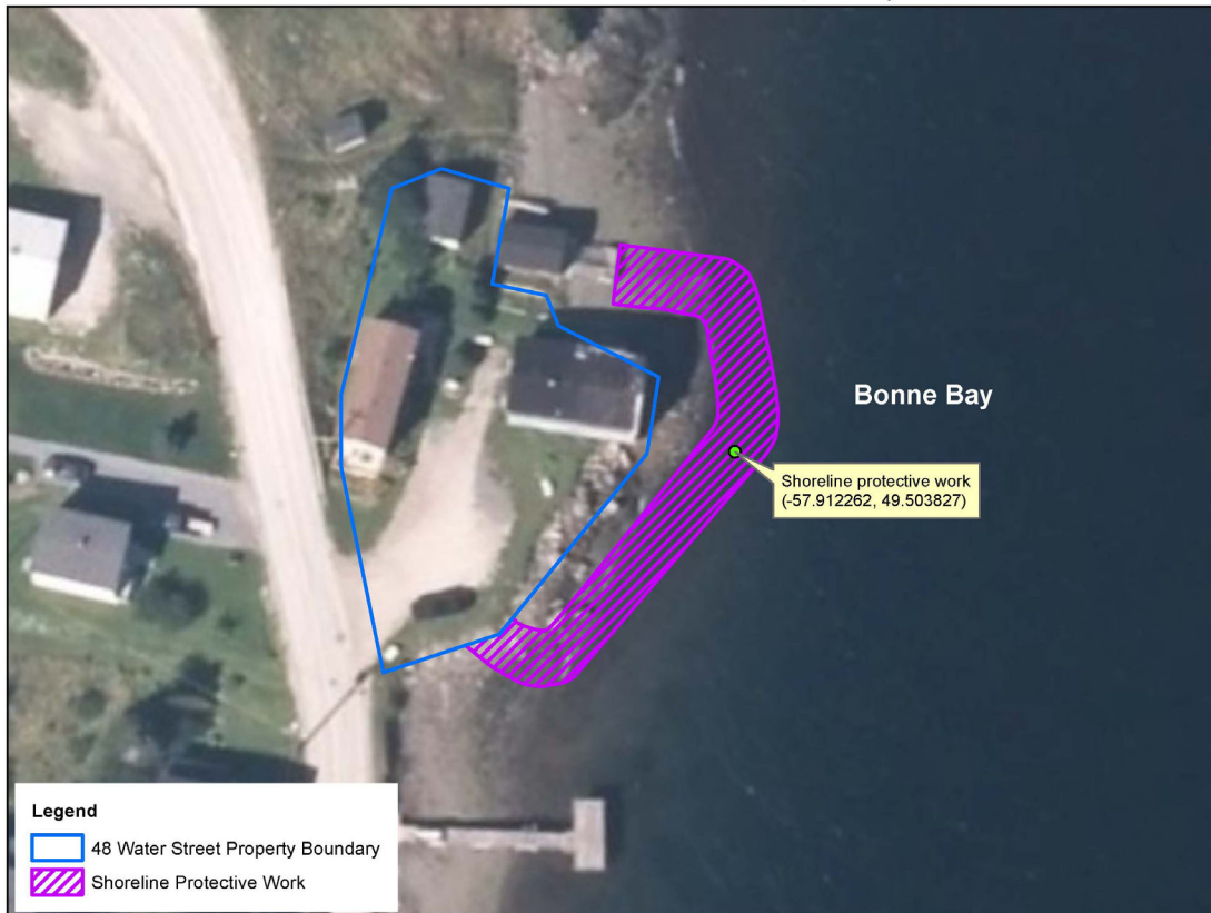
Shoreline Protection Work at 48 Water Street, Woody Point
