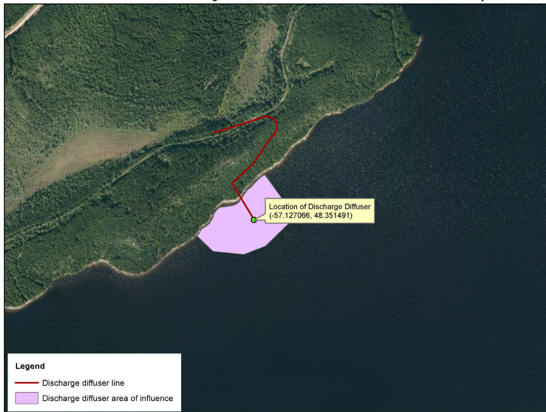
Installation of effluent discharge diffuser into Victoria Lake in Valentine Gold Project
