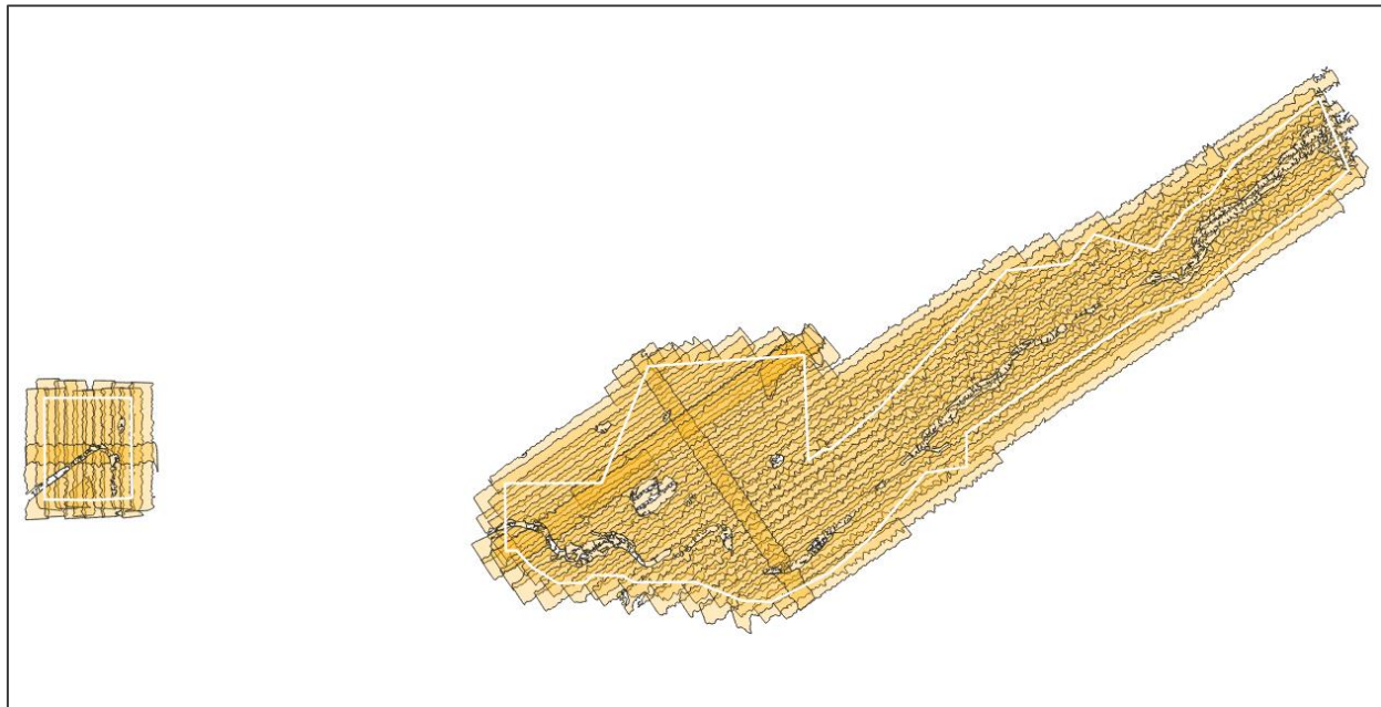
Figure 3. LiDAR collection swaths displayed with transparency, overlaid by project AOI.
