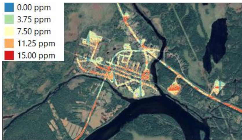
Figure 6. Sample view of density grid of ground points in non-vegetated areas, overlaying satellite imagery of the area.
