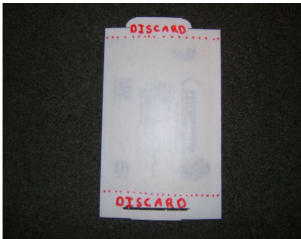
Figure 4. a) Sticky trap showing areas to discard. This border area contains no glue and cannot be used for the snags. b) Cuts to make in order to get the proper sticky pad size. Each pad will be approximately 1 x 2.5 inches.
