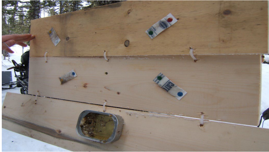
Figure 1. The opened hair trap showing sticky pads (with fur) and sardine can for bait. The top section folds down and the bottom section folds up to form a triangle with the stationary center section which is nailed to the tree trunk. Note placement of sticky pads. Cable ties were used in early work but wire seems to be sturdier and less likely to be damaged by weather conditions.
