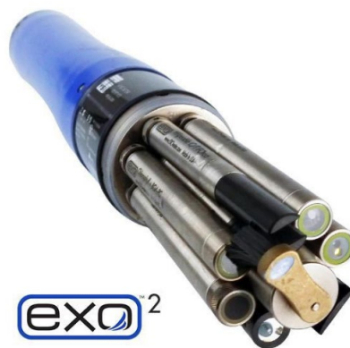
Figure 4: EXO 2 used for monitoring water quality parameters.
