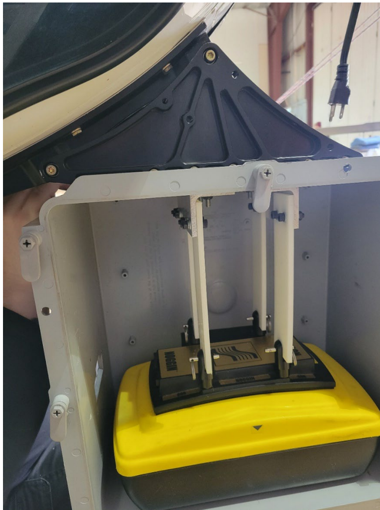
Figure 5. The GPR hardware is mounted inside the enclosure (grey box) using the G1 mount (black angled bracket), to the nose of the helicopter.
