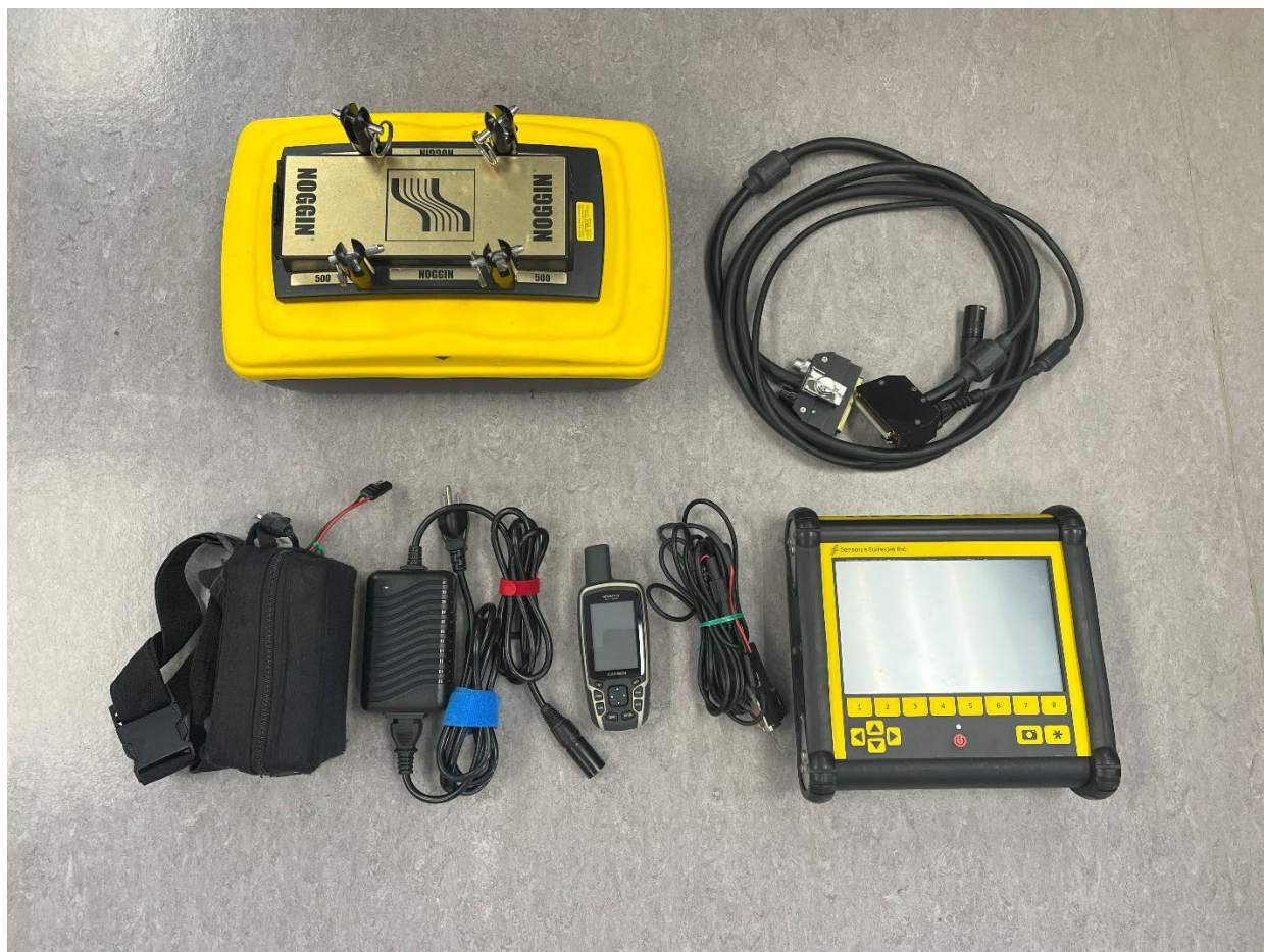
Figure 3. The Noggin 500 system and external GPS used for the helicopter survey. Clockwise from top left, Noggin 500 GPR, power-data cable, Digital Video Logger (DVL) handheld GPS receiver with GPS serial data cable, battery charger and battery pack.
