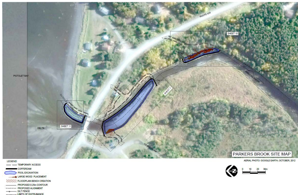
Figure 2. The three areas of proposed pool creation in the lower Parkers River as shown in the preliminary design drawings.
