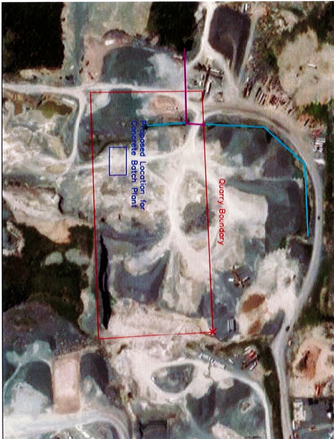
Figure 1: Teal line represents the Drainage ditch that is on the quarry site, and the purple line represents the flow of water through the culvert into the vegetated area
