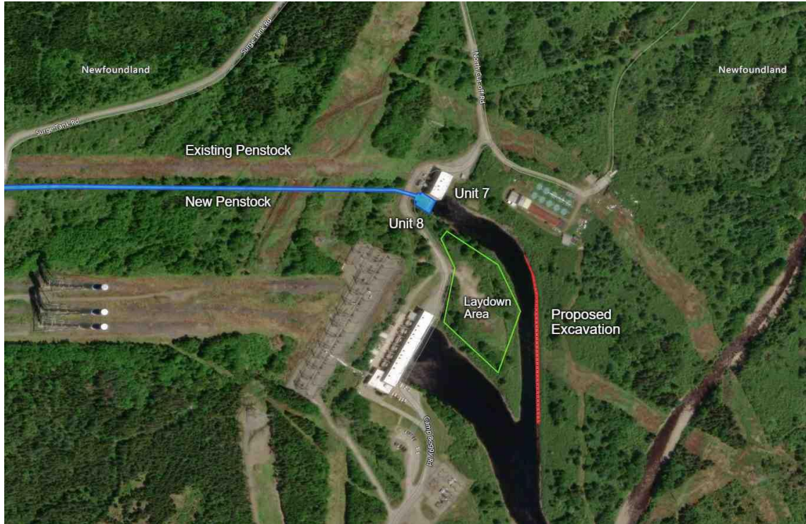
Figure 8-3: Proposed Downstream Components – Tailrace Channel Widening (shown in red), laydown area (shown in green boundary), and location of Unit 8 (shown as blue box)
