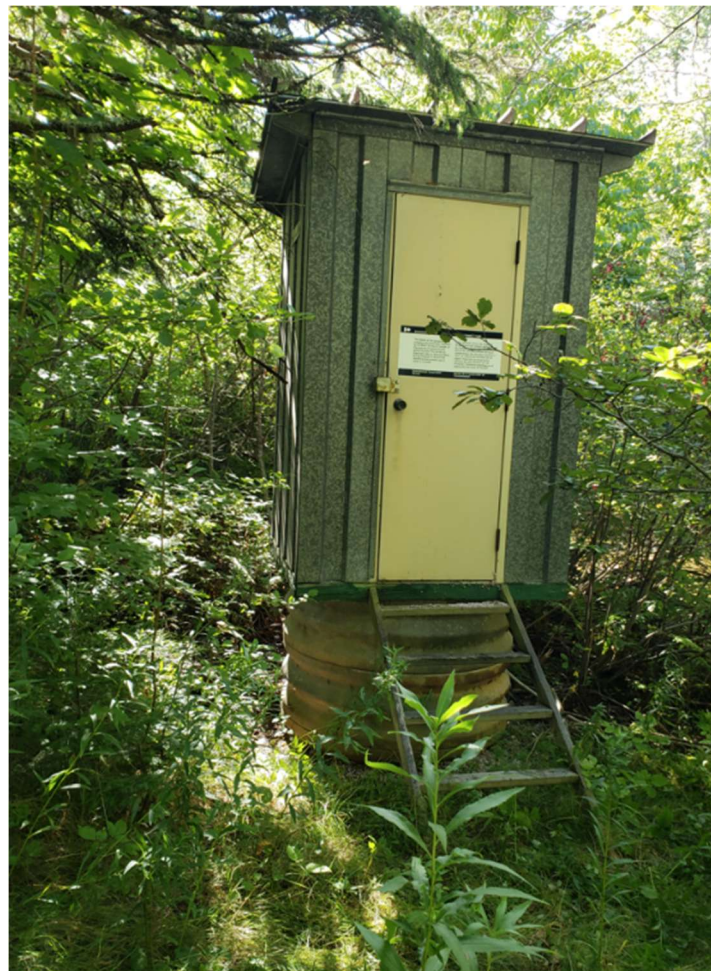
Figure 3. Steel walk-in shelter and stilling well located at 01AP009 Parlee Brook below Arnolds Bridge (Photograph taken September 2, 2022).
