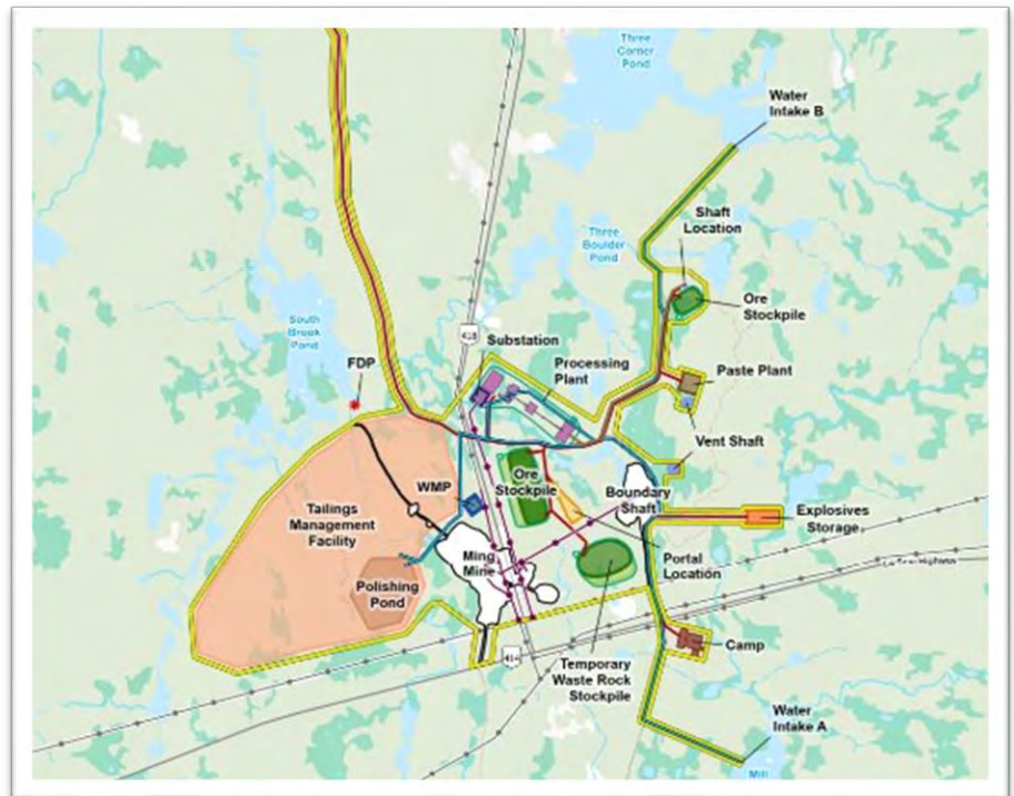
Figure 1: The proposed footprint of the Green Bay Ming Mine Project. It includes a Process Plant (mill and crushing), Tailings Management Facility (TMF), temporary waste rock stockpile, ore stockpile and new accommodations complex for our workforce.
