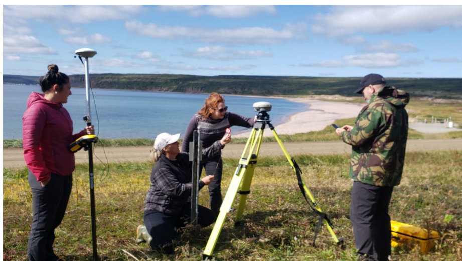
Setting up RTK base station (yellow tripod) at L'Anse Amour.
