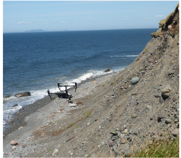
UAV (drone) taking photo of cliff face at oblique angle.
