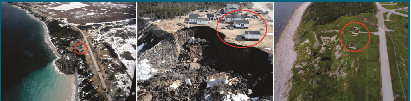
View of the landslide area at Daniel's Harbour shortly after the 2007 landslide (left and centre) and in 2017 (right). Several structures and the road were relocated inland after the landslide. The foundations of the three houses circled in the left and centre photos are circled in the right photo.
