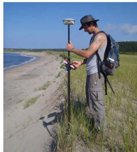
Using an RTK roving receiver at Cheeseman Provincial Park.
