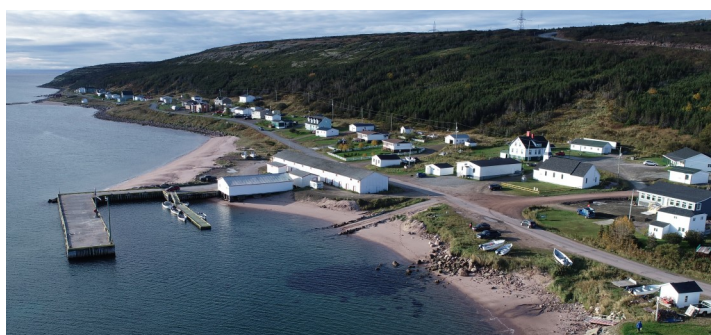
The build-up of sediment behind the wharf in Forteau is evidence of longshore drift. In this example, drift is from the top of the photograph to the bottom.
