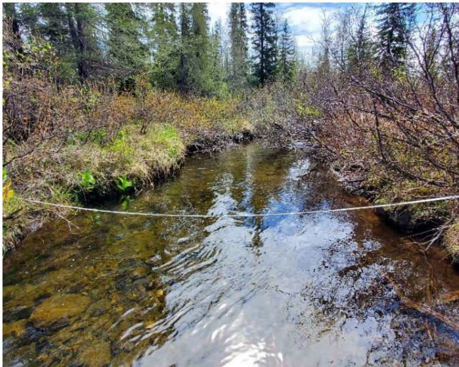
Figure 8-4: A Typical Cross-Section Set-Up for Manual Flow Measurement at a Watercourse
