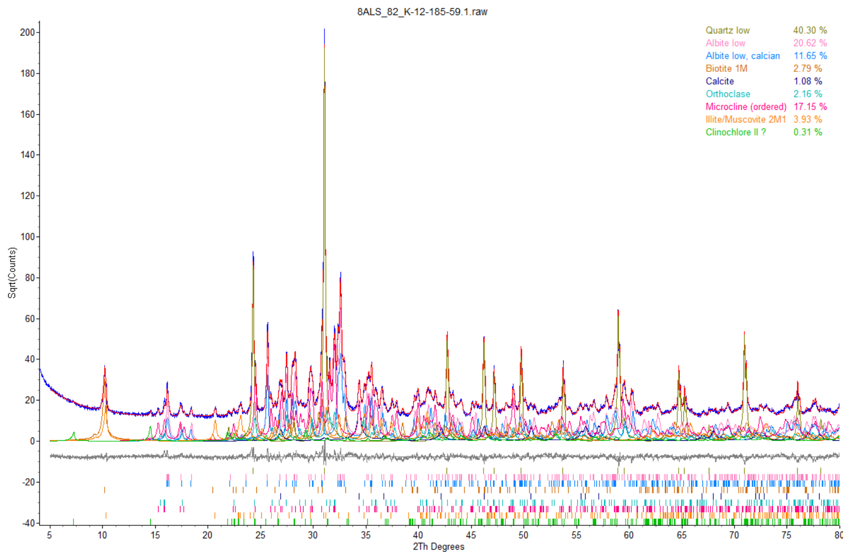
Figure 8. Rietveld refinement plot of sample ALS Geochemistry - 82_K-12-185-59.1 (blue line - observed intensity at each step; red line - calculated pattern; solid grey line below - difference between observed and calculated intensities; vertical bars - positions of all Bragg reflections). Coloured lines are individual diffraction patterns of all phases.
