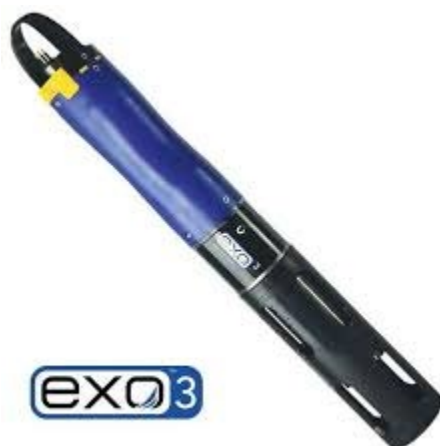
Figure 3. Xylem EXO3 DataSonde used for monitoring five surface water quality parameters.
