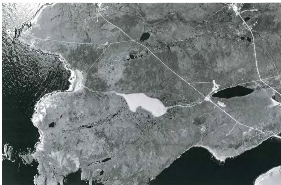
Figure 6.1-17: Aerial Photograph of Shoal Cove Pond (1941), Highlighting Tailings Deposition within the System between Clarke's Pond and Shoal Cove
