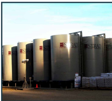
Figure 4-7 Typical Liquid Mud Tank Farm Arrangement
