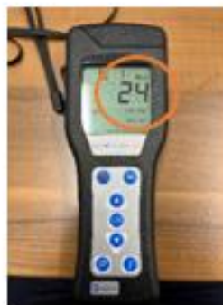
Step 6 – Press 'OK' and system will count down from 15 to give a reading
