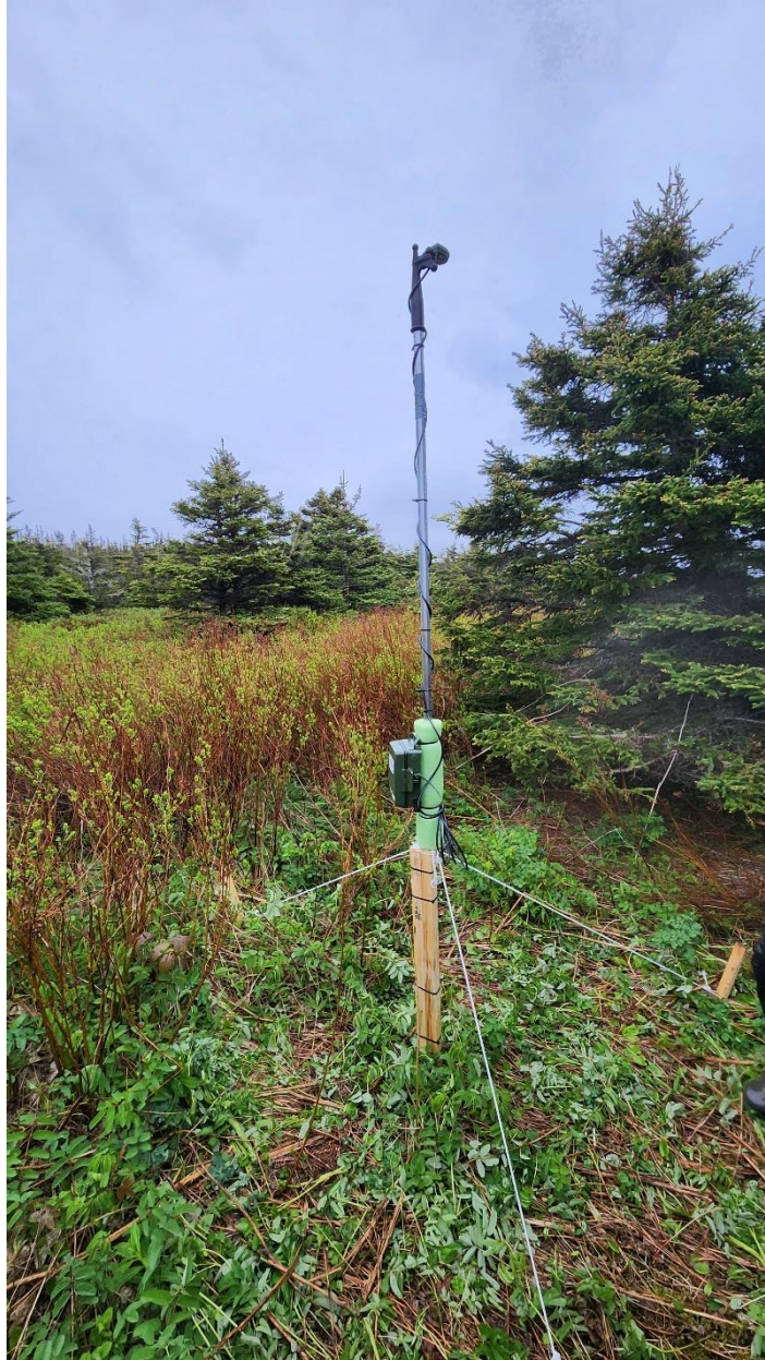
Figure A.1. Example of a deployed ultrasonic bat ARU (Wildlife Acoustics SM4-Bat) attached to a fibreglass pole with supporting guy lines, and its associated microphone mounted at the top.
