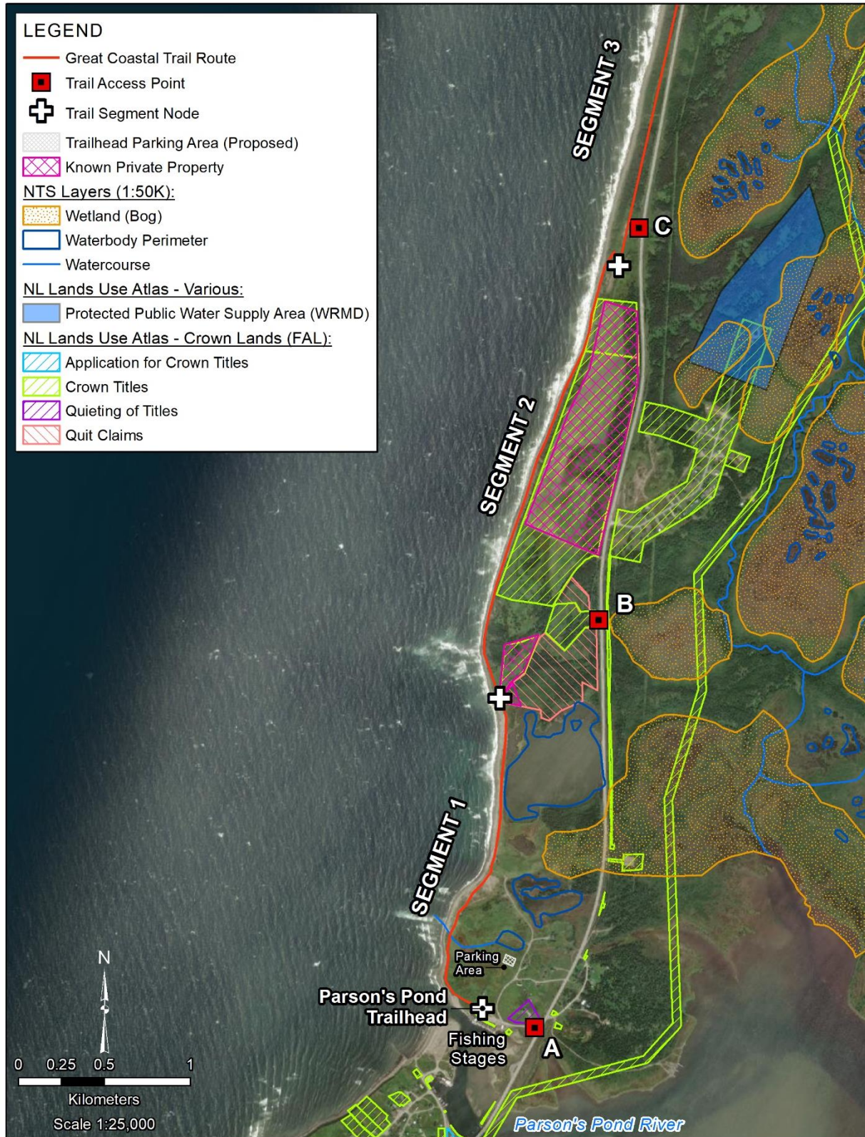
Figure 4.1a. Proposed Great Coastal Trail Project elements (Demonstration Trail Segments 1 to 3, Parson’s Pond) depicting select layers of the National Topographic System (1:50,000 scale) and the NL Land Use Atlas at a scale of 1:25,000.
