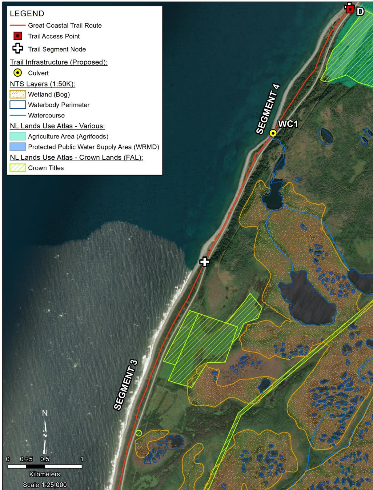
Figure 4.1b. Proposed Great Coastal Trail Project elements (Demonstration Trail Segments 3 to 4) depicting select layers of the National Topographic System (1:50,000 scale) and the NL Land Use Atlas at a scale of 1:25,000.
