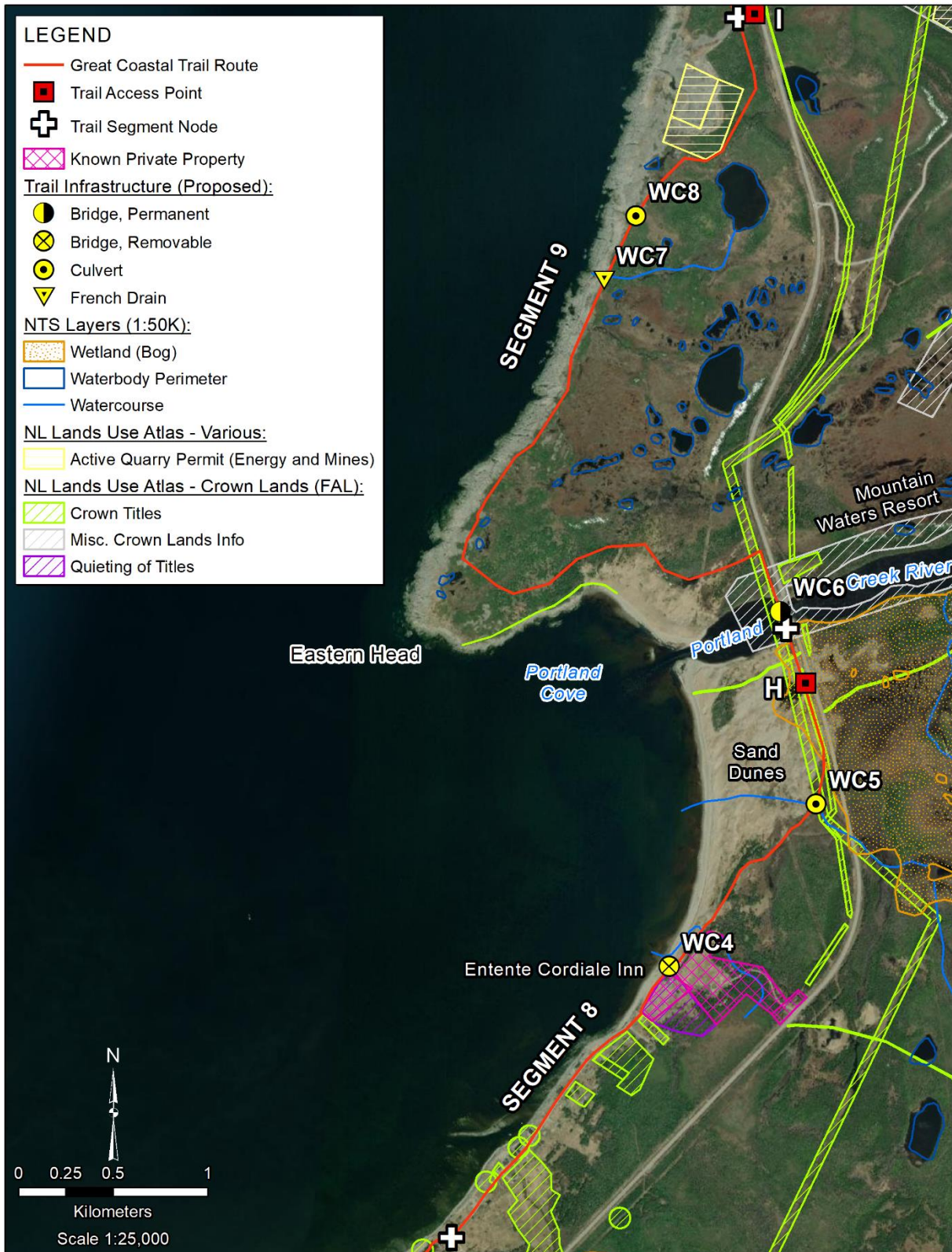
Figure 4.1e. Proposed Great Coastal Trail Project elements (Demonstration Trail Segments 8 to 9, Portland Creek River) depicting select layers of the National Topographic System (1:50,000 scale) and the NL Land Use Atlas at a scale of 1:25,000.
