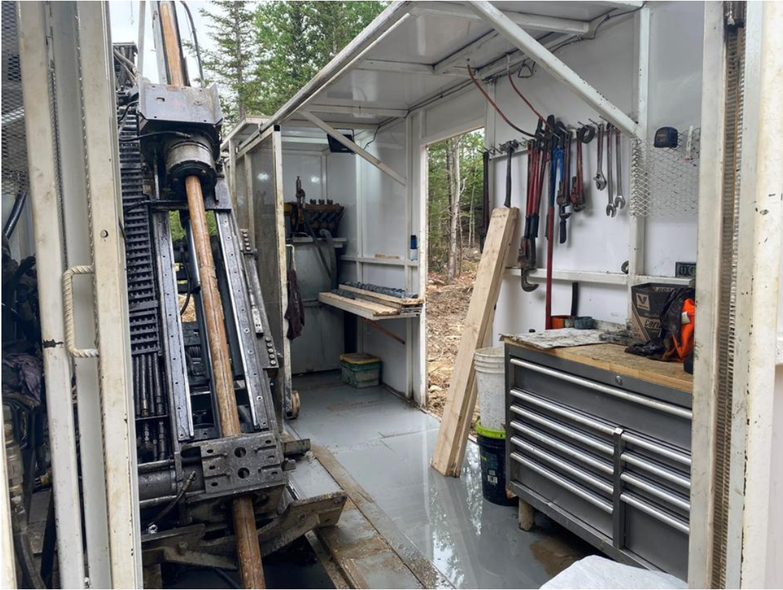
Picture 3: Inside a Typical Diamond Drill Rig.
