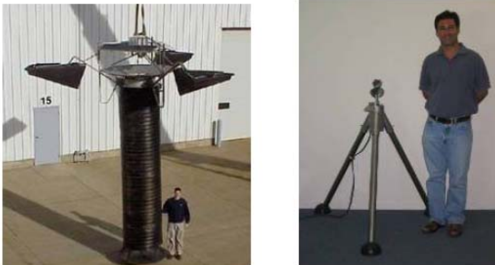
Figure 14: Tank active mixing devices– draft tube (left), vortex mixer (right)
