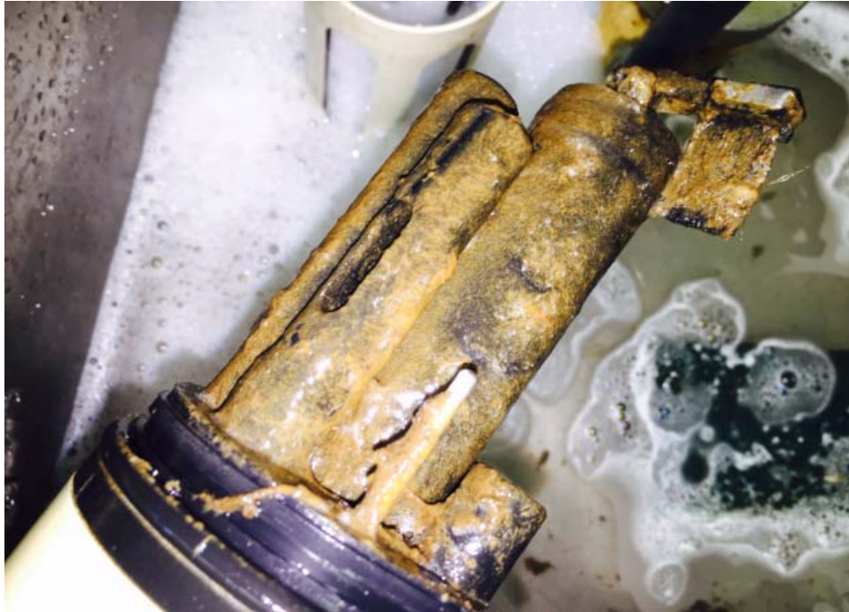
Figure 23: Slime on Airport Water Quality Instrument
