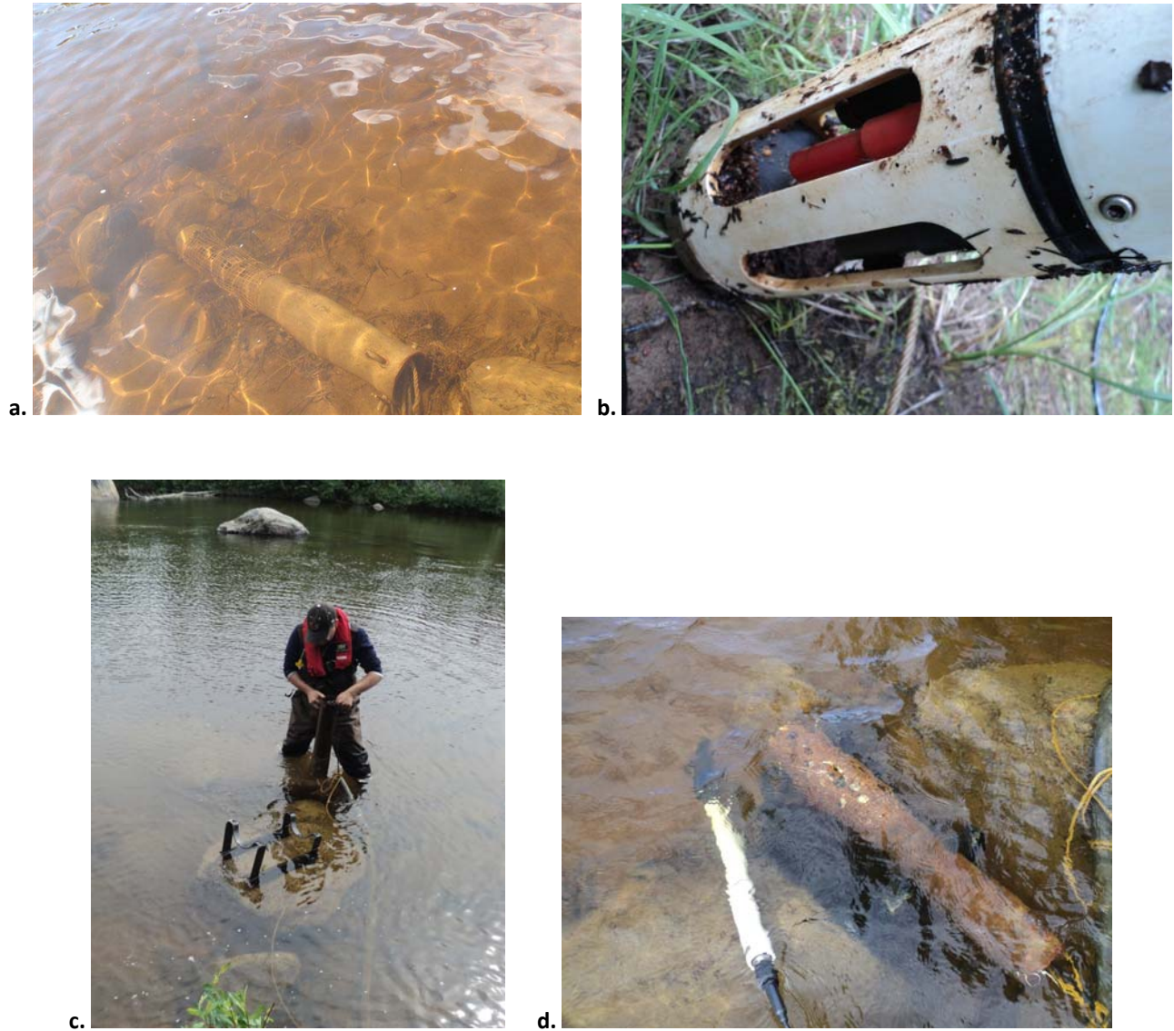
Figure 21: (a) Lower Reid Brook instrument as found by Vale Environment staff during site visit on July 7. (b) Lower Reid Brook instrument as found by ENVC and Vale Environment staff during site visit on July 20. (c) Vale Environment staff installing stand for instrument to prevent rock and debris build up around the instrument sensors. (d) Lower Reid Brook instrument deployed on stand on July 21 (QAQC sonde temporarily deployed for comparison readings).
