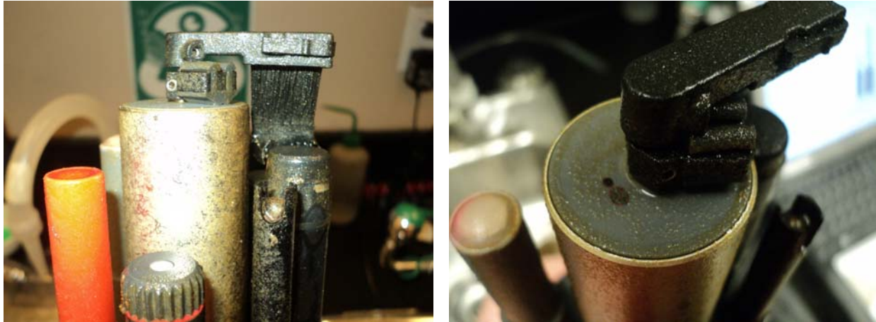
Figure 13: Bio-fouling residue on instrument at Tributary to Lower Reid Brook after wiper and brush failure
