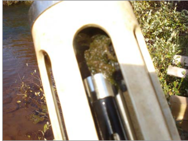
Figure 4. Algae were found on the instrument's sensors at the James Creek station on September 19, 2011, which resulted in poor performance of the turbidity sensor.
