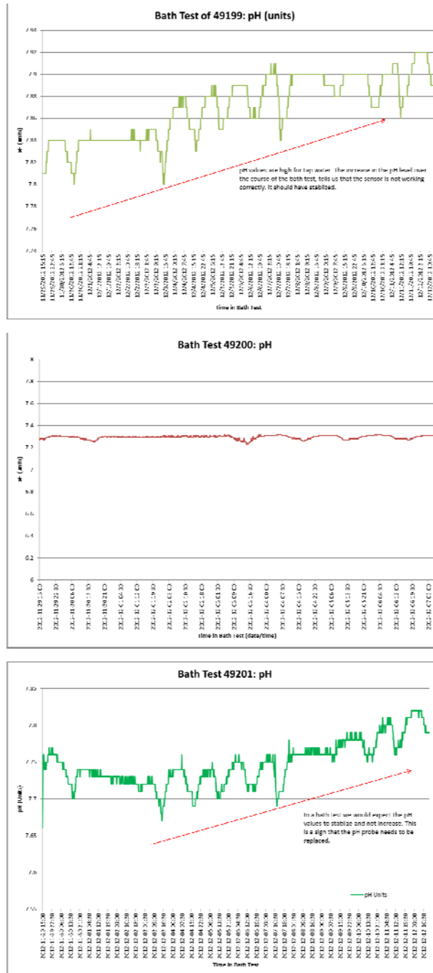
Figure 5. pH data recorded by three instruments during a 14 day bath test, from November 29, 2012 to December 12, 2012. Based on this analysis, it was recommended that pH sensors on instrument 49199 and instrument 49201 be replaced.
