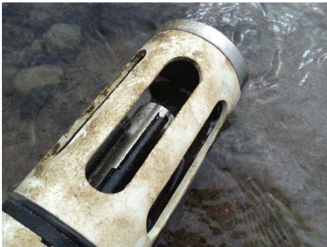
Figure 6: (left and right) Biofouling residue found on instrument at removal on June 29.
