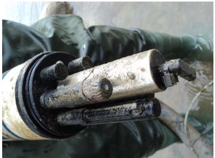
Figure 6: (left and right) Biofouling residue found on instrument at removal on June 29.
