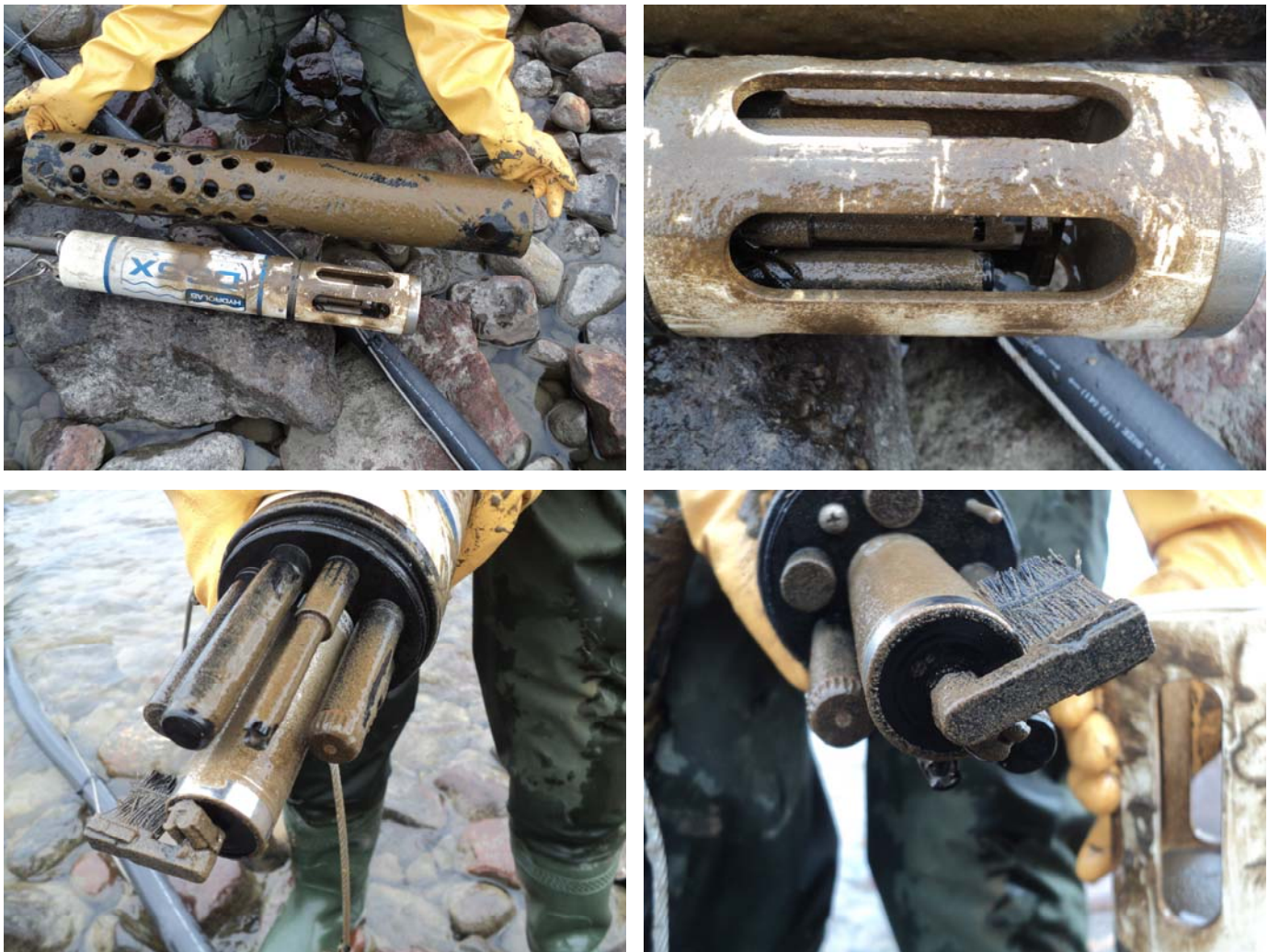
Figure 14: Biofouling residue found on protective casing (top left) as well as on sensor guard (top right), and instrument sensors (bottom left). Turbidity wiper still functioning properly and remove biofouling residue before each reading (bottom right)
