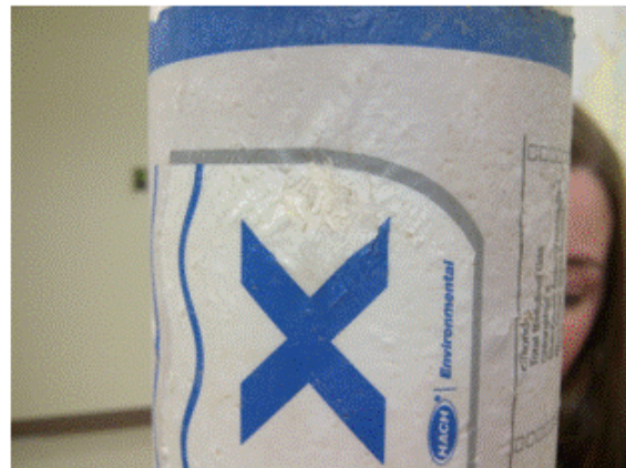
Damage resulting after instrument casing was lost. Hydrolab casing was cracked and dented potentially compromising future use.
