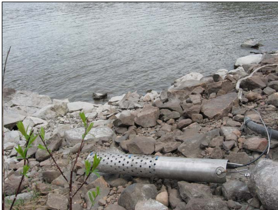
Figure 2: Datasonde within protective metal housing lying exposed to air on the beach at station below Lower Muskrat Falls after stage level dropped significantly in the month of June.
