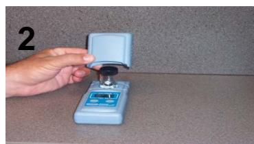
Wipe the bottle and insert into the meter with the diamond facing the keypad. Cover with instrument cap.
