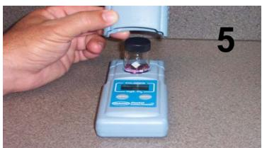
Wipe the bottle and place in the meter with diamond facing the keypad. Cover with instrument cap.
