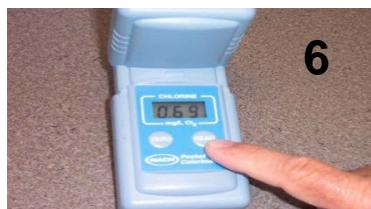
Press READ within 1 minute of adding DPD Free Chlorine reagent. Record results, discard sample, and rinse bottle.
