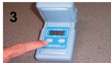
Press the ZERO key; screen will illuminate & show "---" then "0.00". If "0.0" appears, switch meter to low range & repeat Step 3.
