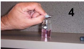
Remove bottle; add reagent from 1 DPD Free Chlorine foil packet; cap bottle and shake for 20 seconds.
