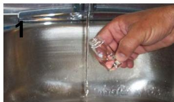
Fill the glass bottle with water to the 10 mL line and cap bottle.
