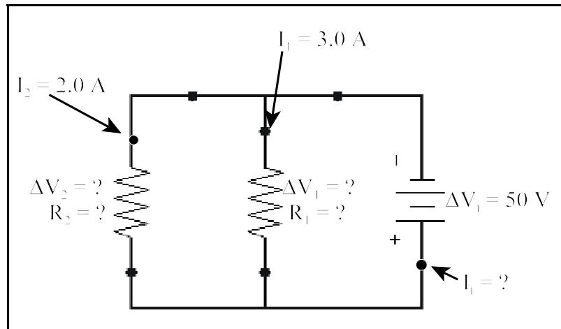
16. In the circuit shown,  $R_1 = 20 \Omega$ . The potential drop across  $R_1$  is 10 V; across  $R_2$ , it is 20 V. Determine the following:
