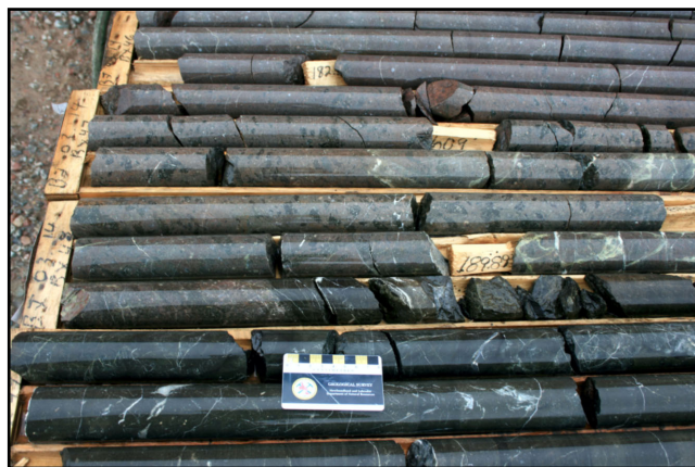
Plate 5. Photo of the lower contact zone of the quartz-feldspar-phyric rhyolite unit and the underlying fine-grained, locally vesicular, mafic volcanic rocks. Note the development of hyaloclastite within the lower 4 to 5 m of the rhyolite unit; DDH BJ-03-014, 190 m depth.
