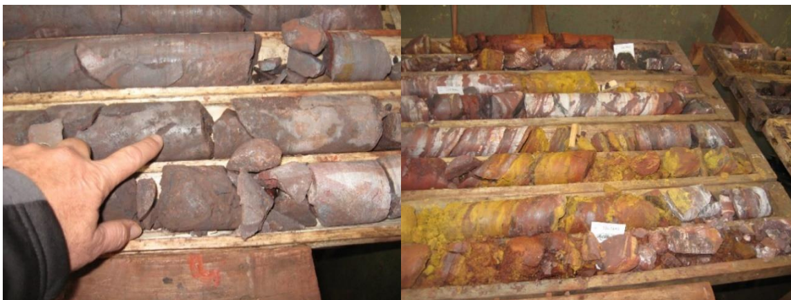
Figure 14-3: Well recovered drill core showing voids at the core shack during site visit October 3-4, 2013
