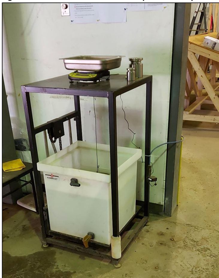
Figure 11—2: 2022 Water Immersion Specific Gravity Station
