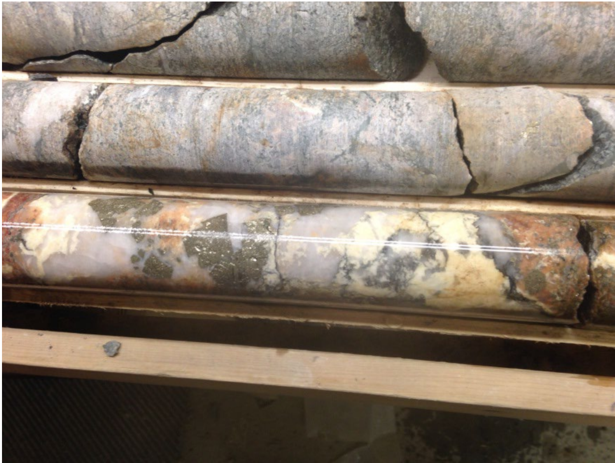
Plate 5: Coarse pyrite within quartz-carbonate vein cutting strongly albitized gabbro (BN-15-217).
