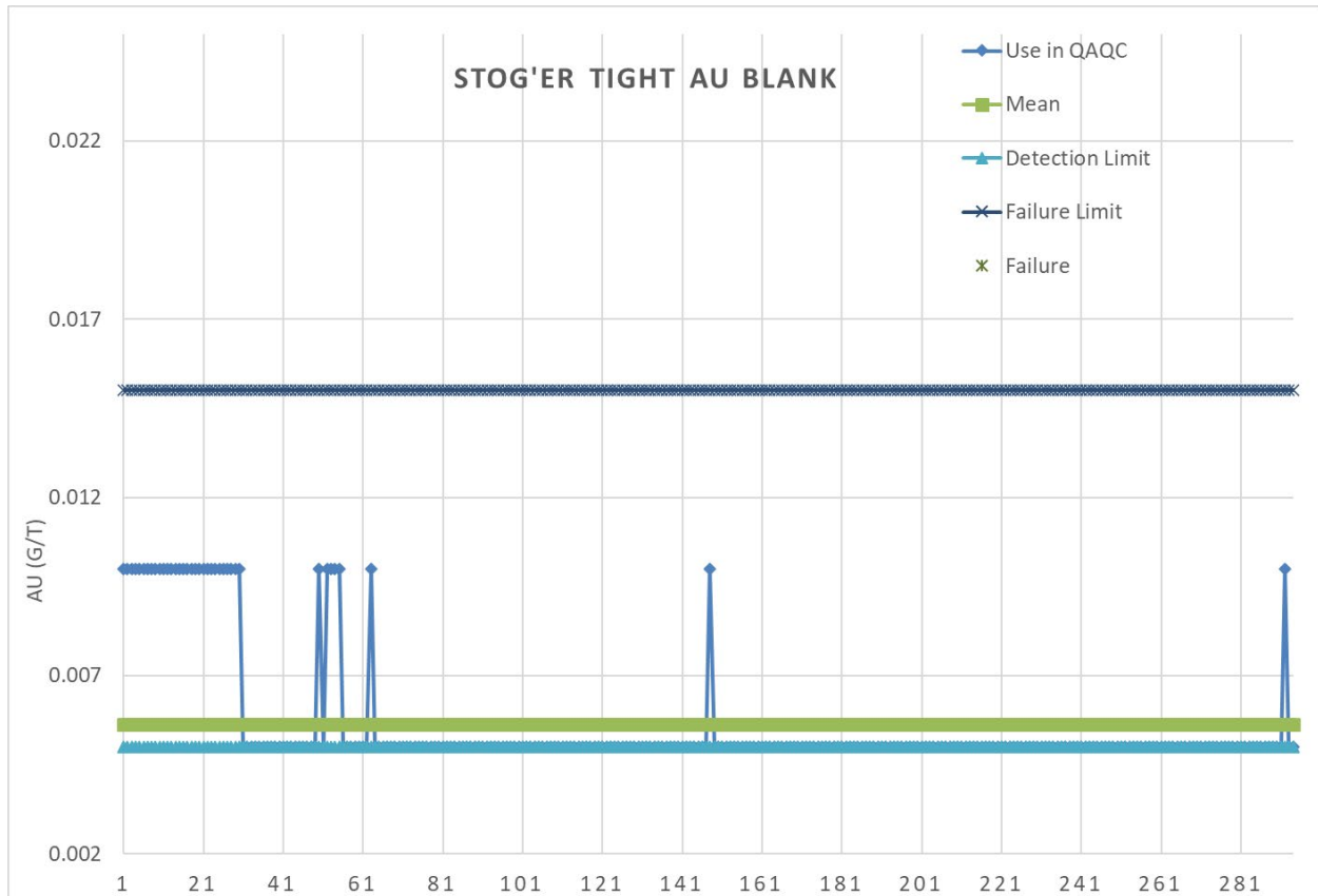
Figure 34: gold (g/t) results for the Stog'er Tight Deposit coarse blanks.
