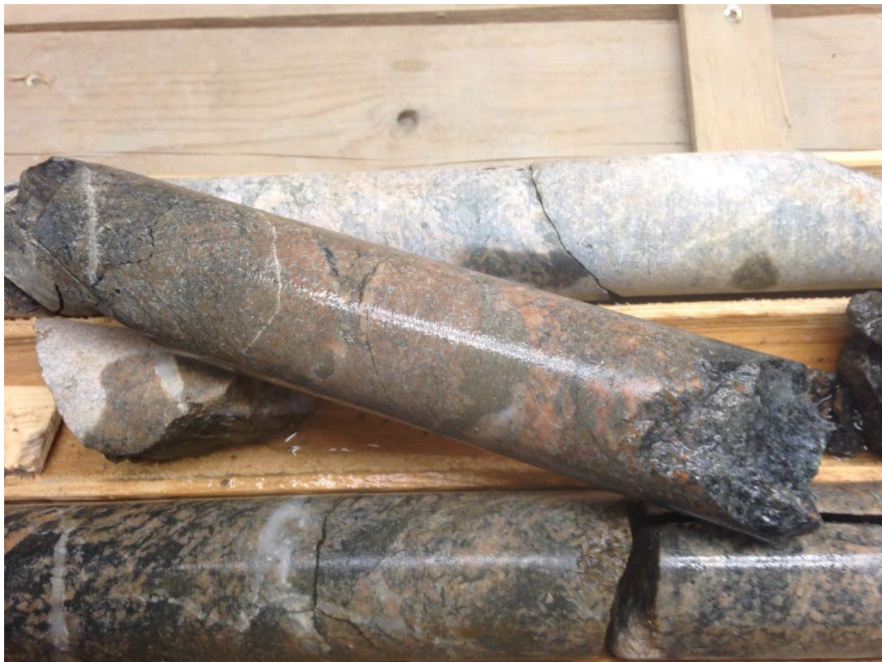
Plate 4: Coarse pyrite associated with quartz veined and strongly albitized gabbro, (BN-15-217).
