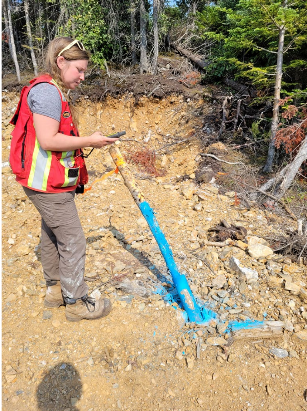
Plate 12: Drill collars pickets outlining the drill hole name, azimuth, and dip.
