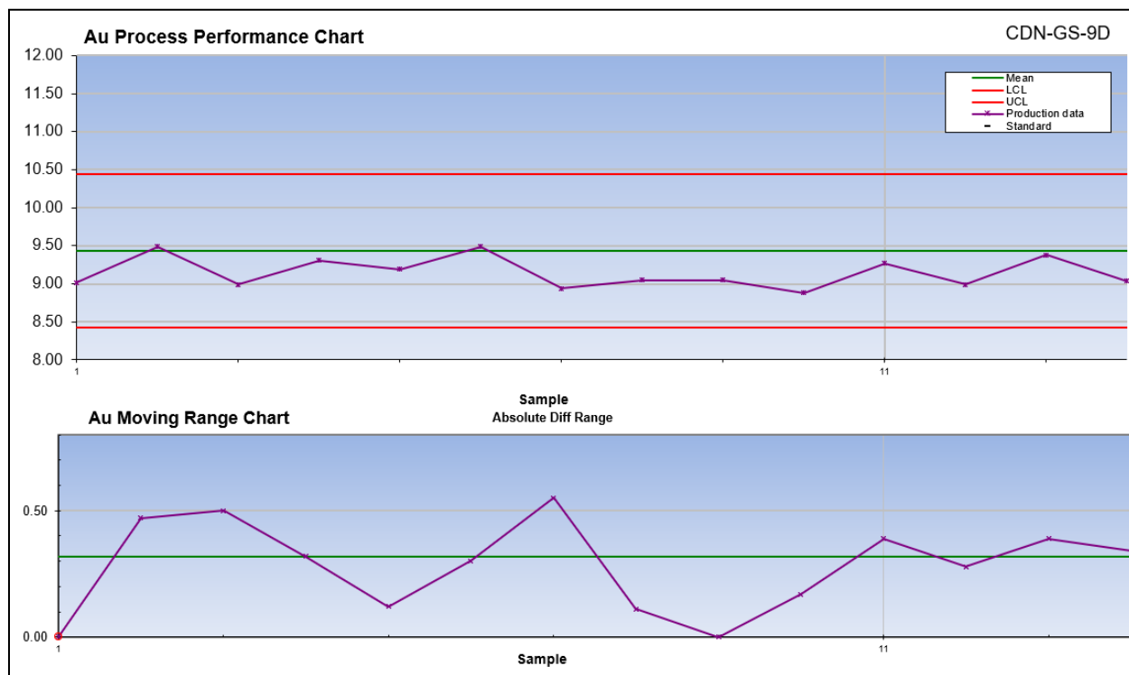
Figure 33: Stog'er Tight Deposit Standard CDN-GS-9D gold (g/t).
