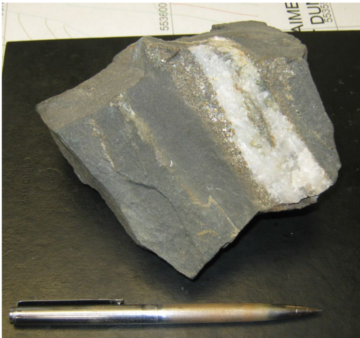
Plate 6: Grab sample from Goldenville Mine Dump showing coarse pyrite mantling quartz veining developed within magnetite-rich iron formation.
