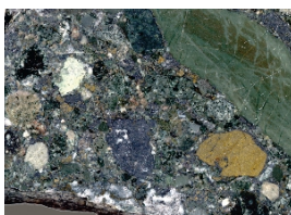
Zn-Pb-Cu breccia (transported) ore with clasts of massive sulphides (Buchans Mine)
