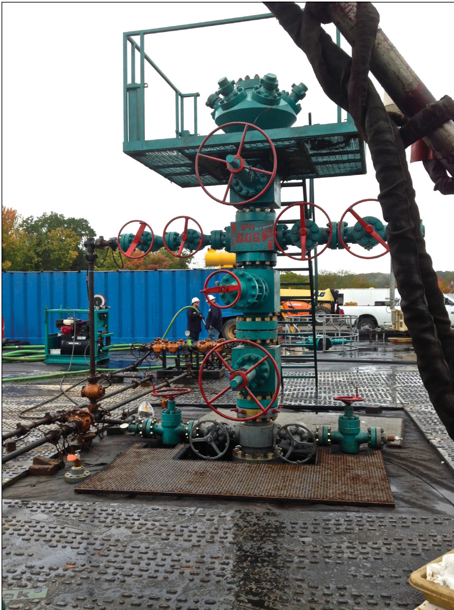
Figure 10. Wellhead ready for hydraulic fracturing.
