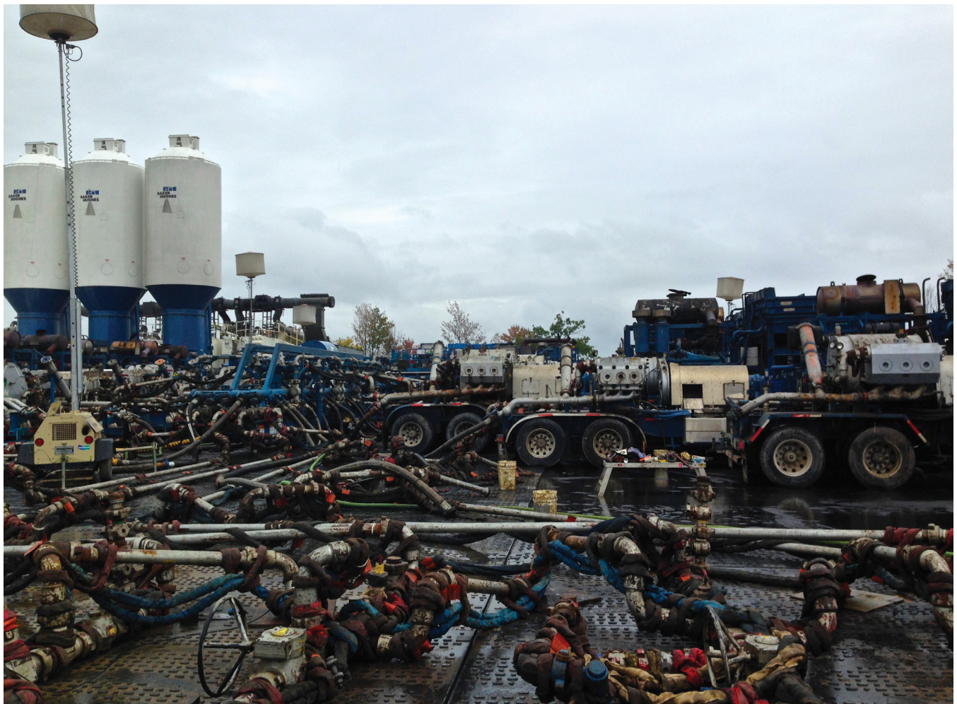
Figure 12. Pumping trucks and other equipment on well pad.
