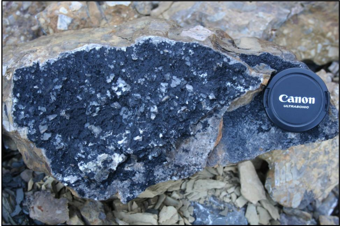
Location 8: Hydrocarbon stained fracture surfaces within parted limestones of the Cow Head Group; at Portland Creek Quarry. Larry Hicks (DNR) photo
