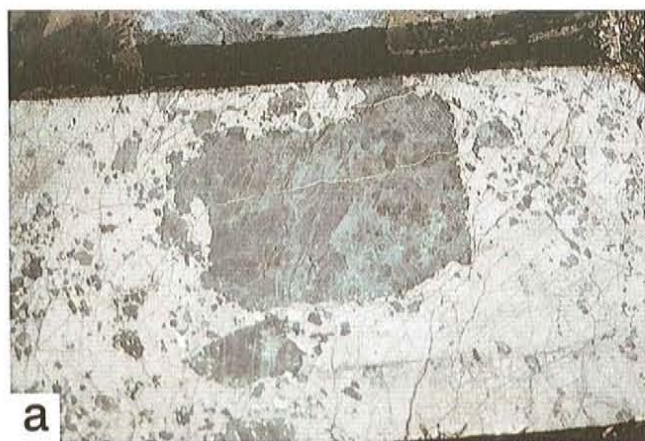
Plate 3. Sulphide zones from the Canadian States Resources License 1514 prospects. a) Massive sulphide containing multicrystal fragment of wall-rock anorthosite, itself cut by earlier chalcopyrite veinlet. G-zone surface showing. b) "Pseudo-network" texture, where chalcopyrite appears to have percolated and eroded along grain boundaries in the wall rocks prior to arrival of nearby massive pyrrhotite zone. G-zone surface showing. c) Vein of massive sulphide containing coarse chalcopyrite and pentlandite, cutting through large plagioclase crystals in wall-rock anorthosite. E-zone, drillhole 1514-96-21. Drillcore in (a) is approximately 12 cm wide; other cores are approximately 4 cm wide
