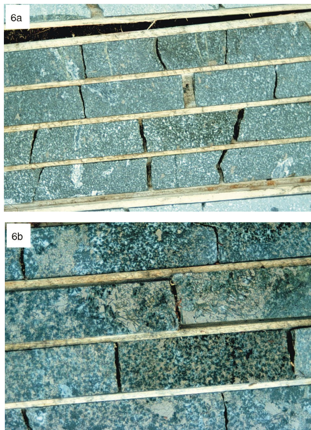
Plate 6. Mineralized rocks from the South intrusion. (A) Melagabbro to peridotite containing minor interstitial sulphides and gneissic fragments, seen as white patches. (B) Gabbroic unit containing magmatic sulphide mineralization and showing well-developed interstitial sulphide textures.
