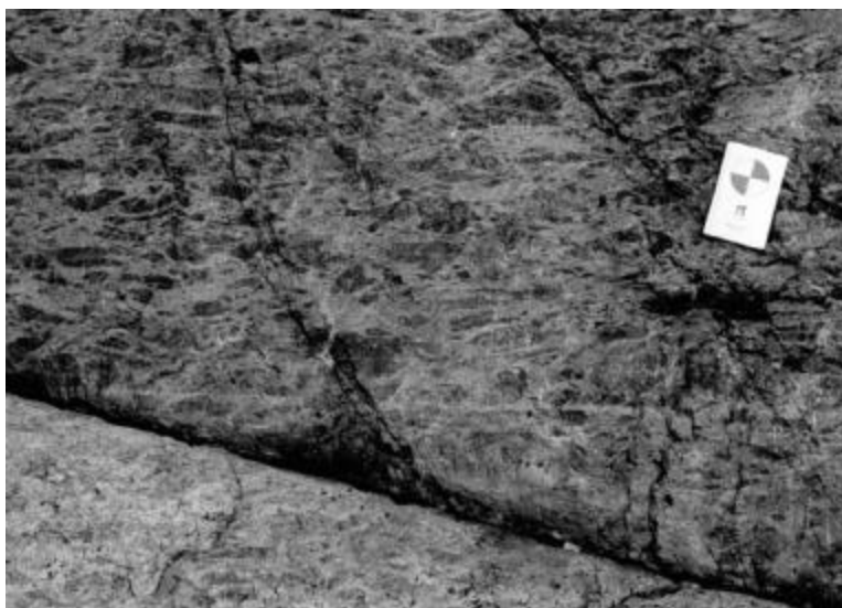
Plate 4. Dark-grey, fractured, oriented, igneous plagioclase remnants in a granular recrystallized matrix, within anorthosite of the marginal zone of the Mount Lister intrusion, shore of Conch Bay.
