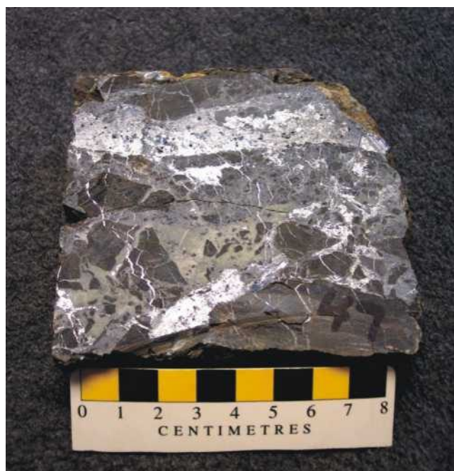
Plate 13. Beaver Brook (Hunan or Central zone) antimony prospect: Quartz–carbonate veins thought to be of epithermal character, crosscut fault-brecciated sedimentary rocks of Davidsville or possibly Badger groups.
