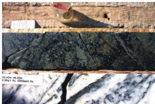
Plate 3. Golden Promise prospect (Jaclyn zone): Drill core illustrating spotted, light green (quartz-sericite-carbonate) and dark green (chloritic ?) alteration in fine-grained parts of the host sedimentary rocks to the Jaclyn vein.
