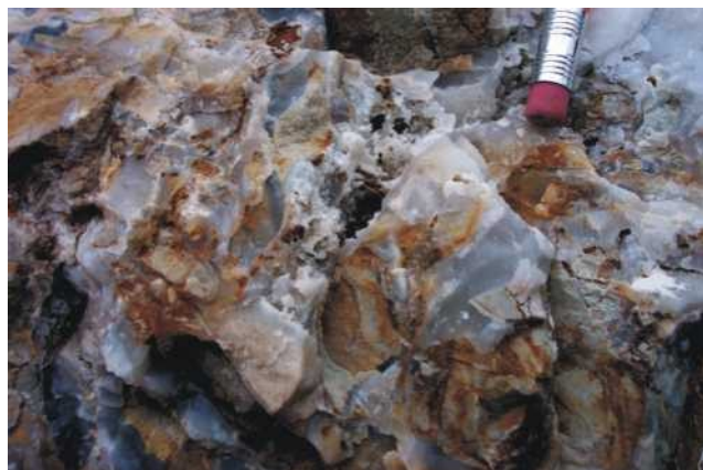
Plate 11. O'Reilly showing: The banded chalcidonic quartz matrix to a tectonic siltstone breccia in probable Silurian rocks, demonstrates the epithermal nature of this showing.
