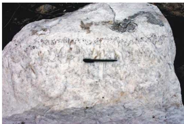
Plate 2. Golden Promise prospect (Jaclyn zone): Boulder illustrating 'caterpillar track' texture, a feature caused by growth of parallel quartz crystals, between which some of the gold has precipitated. Black circles mark areas of visible gold.
