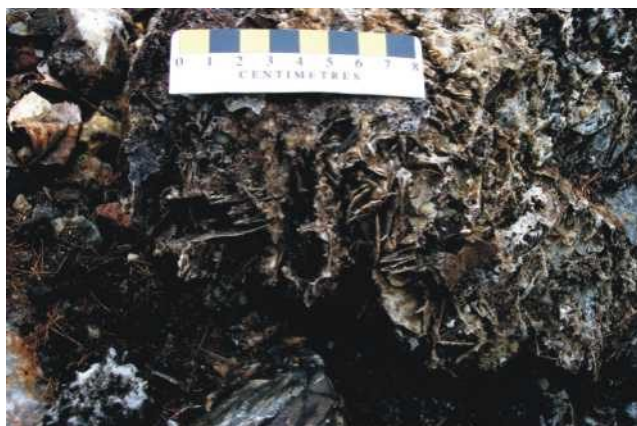
Plate 8. Barite zone showing: Bladed texture of barite in this area may be indicative of precipitation in an epithermal environment.
