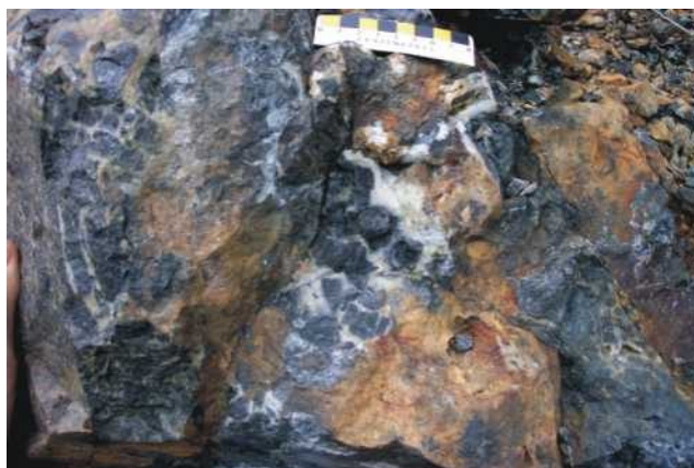
Plate 6. Mustang prospect: Silicification and quartz-veining of low-sulphidation epithermal character in siliciclastic sediments of the Davidsville Group.
