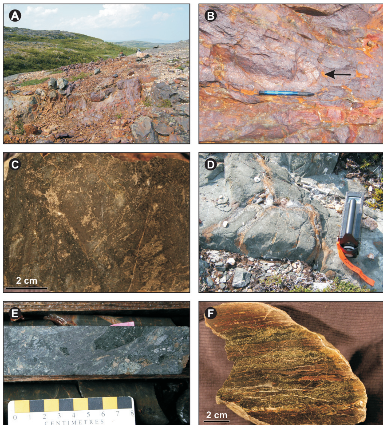
Plate 5. Representative photographs showing typical features of uranium mineralization and associated host rocks at the Kitts deposit and Nash prospect. A) Surface outcrop of the A-Zone at the Kitts deposit; the gossan zone, which hosts the uranium mineralization, is approximately 5m in width, and is bounded by metagabbro to the left and deformed pillow basalt to the right. B) Sulphide-rich metasedimentary rock that hosts uranium mineralization at Kitts; note fold defined by sulphide band at centre of photo. C) Polished sample of uranium-bearing metasedimentary rock from the Kitts A-Zone, showing abundant sulphides and strong deformation. D) Pillow structures that are locally preserved within mafic volcanic rocks adjacent to the Kitts deposit. E) Mineralized drill core showing debris-flow textures that are locally preserved within the host metasedimentary rocks at the Kitts deposit; note abundant sulphides. F) Polished sample of strongly deformed mineralized metasedimentary rocks at the Nash prospect.
