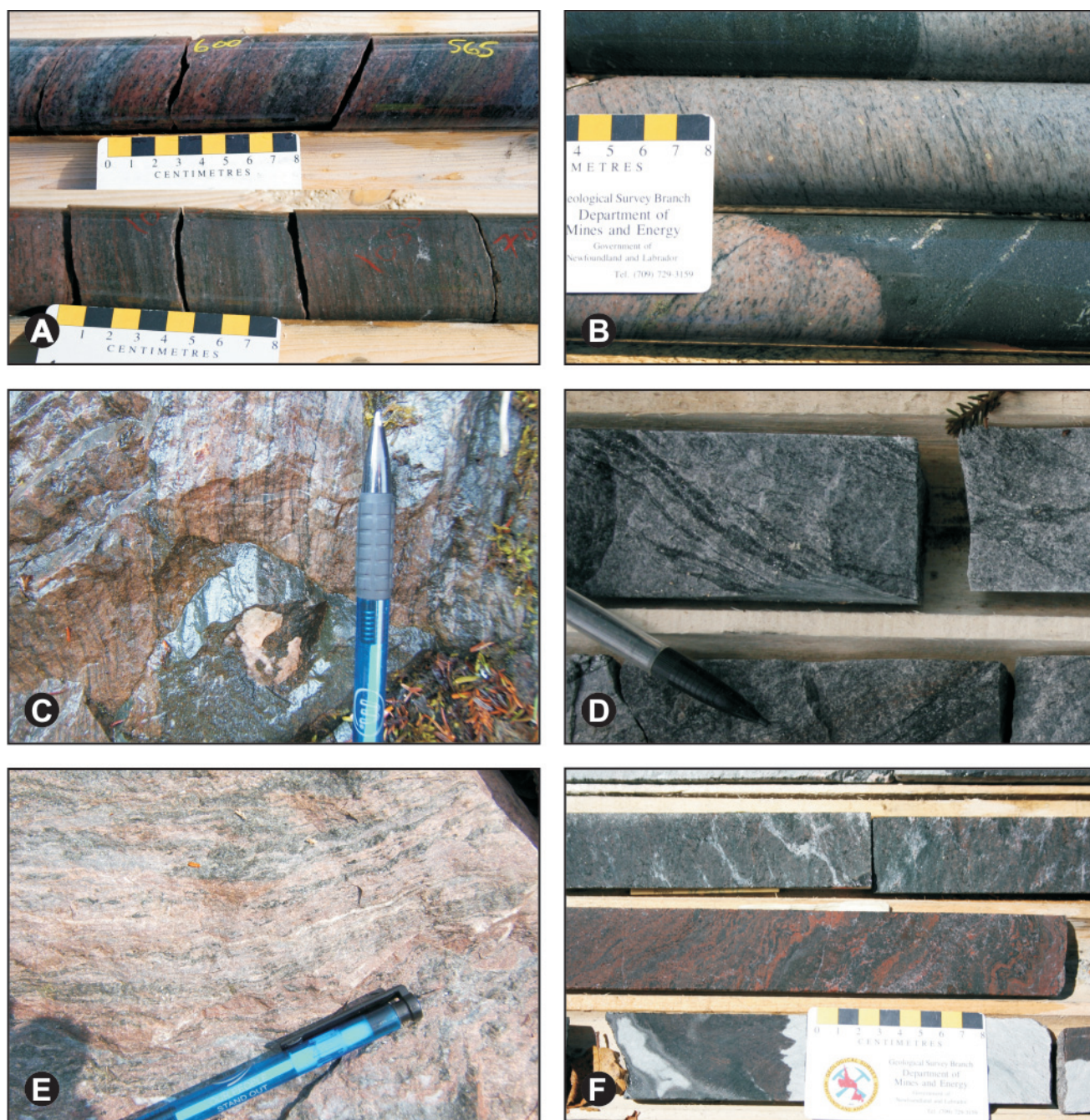
Plate 4. Representative photographs showing typical features of disseminated uranium mineralization hosted within felsic metavolcanic rocks of the Aillik Group. A) Strongly foliated mineralized felsic metavolcanic rocks showing variable degrees of hematite alteration, Michelin deposit. B) Foliated felsic volcanic rocks cut by a mafic dyke interpreted to be of post-mineralization and post-deformation timing, Michelin deposit. C) Outcrop of the strongly foliated, mineralized felsic to intermediate metavolcanic host rocks to the Jacques Lake deposit. D) Mineralized core from the Jacques Lake deposit showing distinctive biotite-actinolite bands (veins ?) that are locally associated with uranium mineralization. E) Strongly deformed, mineralized felsic metavolcanic rocks at the Aurora West prospect, located in an inferred regional shear zone approximately 12 km southwest of the Jacques Lake deposit. F) Strongly deformed felsic metavolcanic host rocks showing intense hematization associated with uranium mineralization (at centre of photo), Mustang Lake prospect, 9 km northeast of Michelin. Light and dark areas in the lower part of photo indicate dry versus wet core and have no geological significance.
