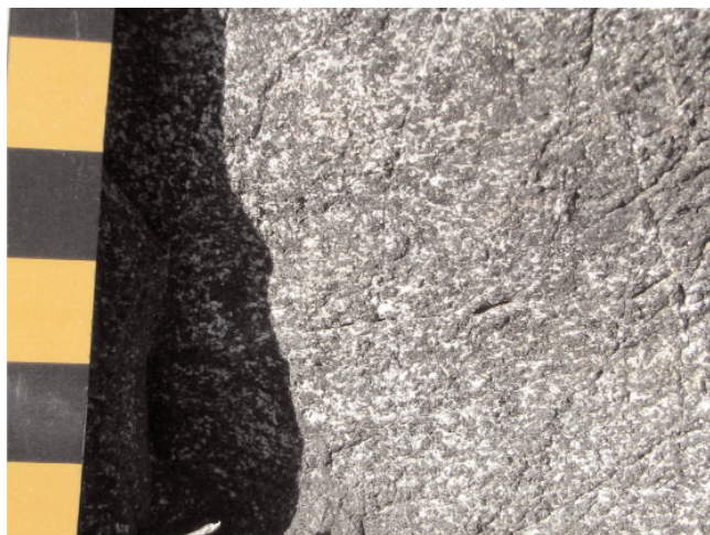
Plate 4. Representative photograph of the pre-1860 Ma Kitts metagabbro (Unit 15), which is composed of recrystallized amphiboles (tremolite to actinolite) but retains a relict igneous texture.
