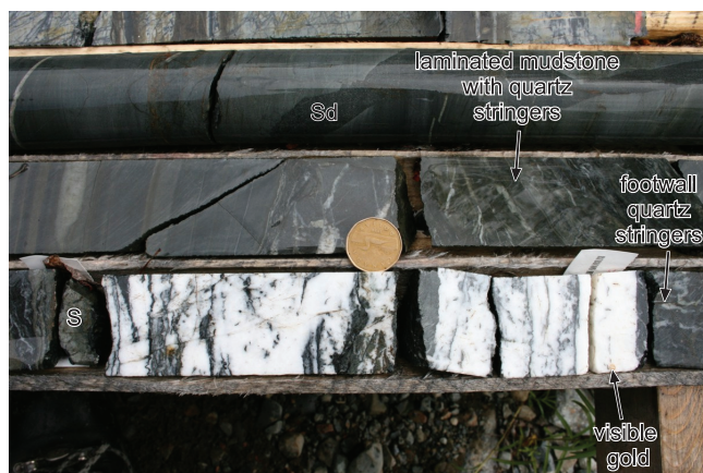
Plate 5. One of the major, bedding-parallel, auriferous quartz veins intersected by drillhole GP07-76. The vein is ca. 25 cm in width, occurs at a depth of 123.1 m and yielded an assay of 0.51 g/t Au and 1479 ppm As. Note the stylonitic texture of the vein and, in particular, the abrupt lower margin of the quartz vein and a series of perpendicular quartz stringers in mudstone in the footwall. Top of hole is to the top left of photograph. The coin is 26 mm in diameter.
