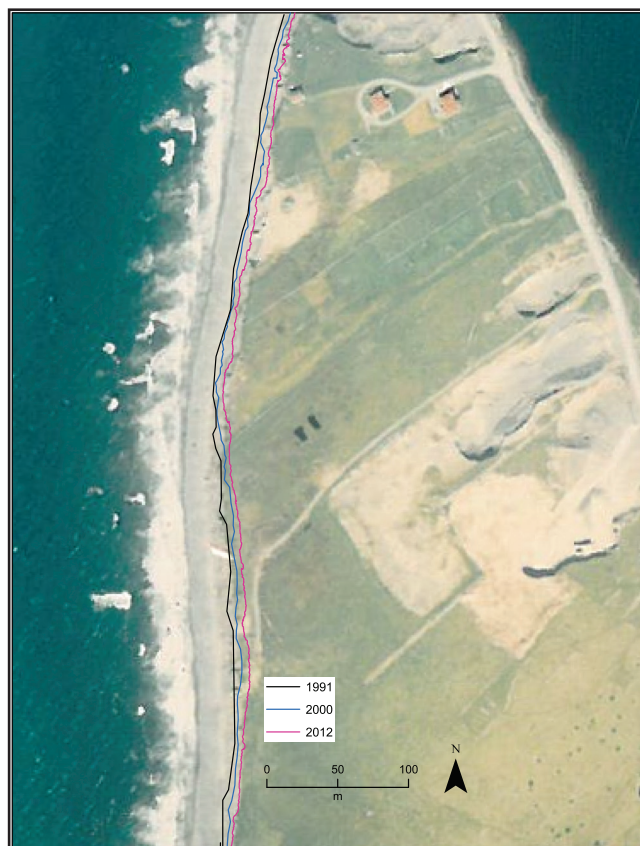
Figure 5. Location of the cliff-top position at Point Verde in 1991 (black), 2000 (blue) and 2012 (red) superimposed on an airphoto. The gravel pit has expanded and is now within 10 m of the cliff edge.
